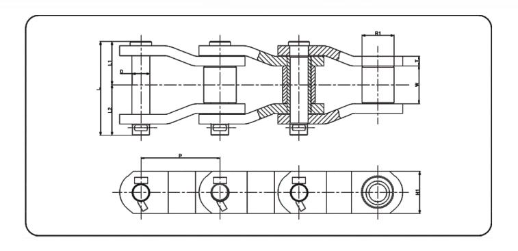
The heavy duty offset sidebar roller chain is designed for drive and traction purposes, and is commonly used on mining equipment, grain processing equipment, as well as equipment sets in steel mills. It is processed with high strength, impact resistance, and wearing resistance, so as to ensure safety in heavy duty applications.
